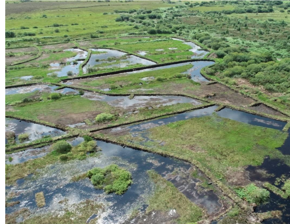
Cell bunding on cutover bog at All Saints Bog . SAC. Carried out by BnM for NPWS
